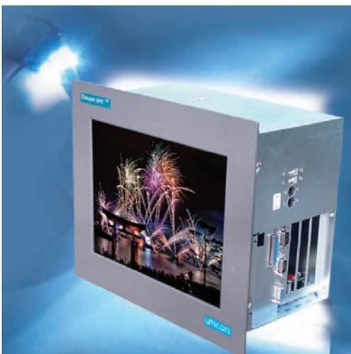
Uticor Power or Tough IPC is an ideal platform not only to run Uticor's soft HMI application (UtiSoft), it is also the perfect plant floor computer to monitor and control the entire plant floor that has Uticor's Toughpanels or Tough TouchPLCs.
