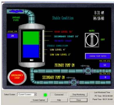
With UT-NVC software installed in your PC you could monitor any screen on the Touchpanel addressed by the software in Real-Time allowing system troubleshooting and/or management review of the machine operation.
