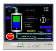
With UT-NVC software installed in your PC you could monitor any screen on the Touchpanel addressed by the software in Real-Time allowing system troubleshooting and/or management review of the machine opertaion.
