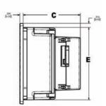
A - Panel Width, B - Panel Height, C - Maximum Product Depth is 4.5" for 4", 6", 8", 10", & 6" depth for 15" unit
